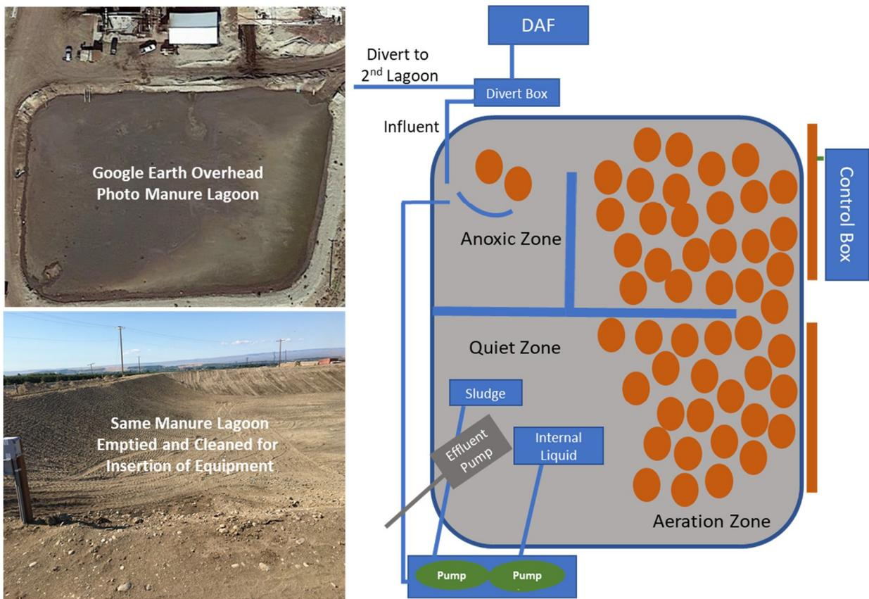
Figure 3. Photos and schematic of NDN lagoon and NDN system: (a) overhead image of existing storage lagoon to be converted to NDN system; (b) photo of that same lagoon after being emptied, cleaned and prepped for equipment insertion; (c) how the existing lagoon is divided into active NDN quadrants with appropriate NDN equipment (orange are submerged micro-aerators, thick blue lines are floating baffle curtains)
