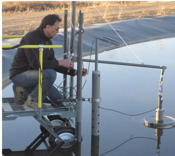
Larry Johnson, NRCS State Engineer giving a final check of the Delta Probe Seepage Meter System to begin recording data.
