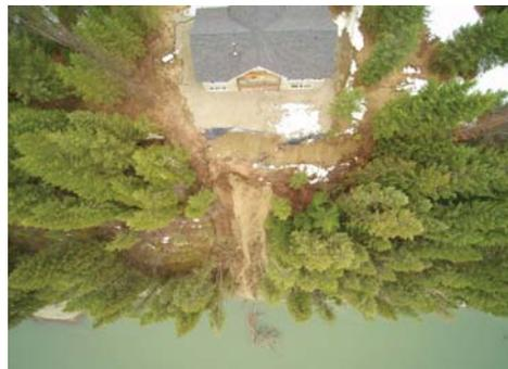
Mass bank failure in Lone, WA on the Pend Oreille River, Spring 2017. Photo: Landowner drone footage
