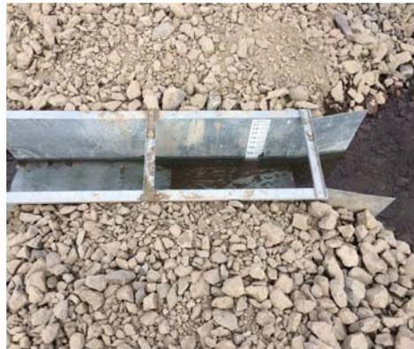
Aquifer recharge flow measurement flume.
