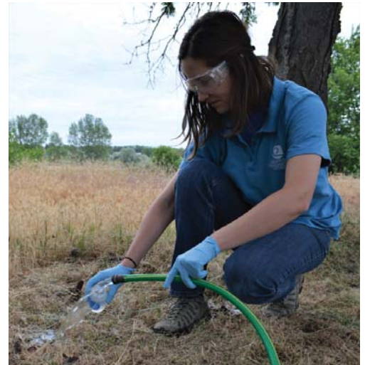
BCD resource conservationist collects water sample from a private drinking well for free nitrate testing. Photo by Rachel Little
