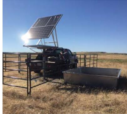
This solar panel can be rotated seasonally to follow the sun, and the watering tank is designed to reduce ice buildup.
